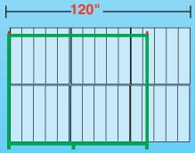
Designing with a fixed or rigid material such as corrugated plastic pigeon holes, would require an OD of 120" x 47.5" x 73.25". This would not fit length way into a standard truck trailer. Our hanging bag OD is only 89.5" x 47.5" x 73.25".
