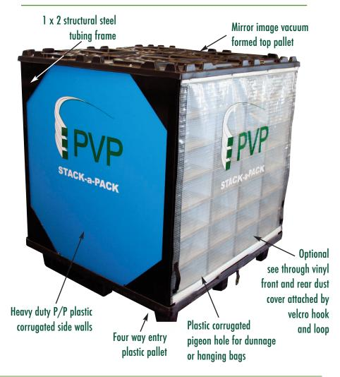
**Product Features:** constructed using a standard 45x48 AIAG pallet and interlocking cap combination with rugged 1x2 structural steel frame construction with heavy duty polypropylene plastic side walls ● the PVP Stack-A-Pack can be prototyped and manufactured more quickly than traditional metal racks ● supplied with either custom plastic corrugated pigeon hole dunnage or returnable hanging bag system.
